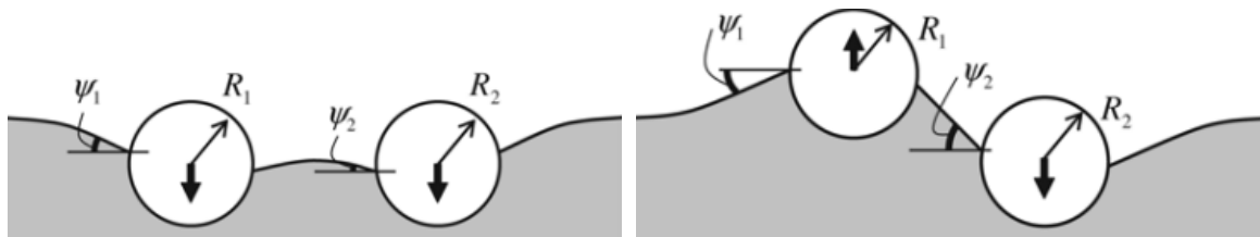
Figure 1. Interactions between two particles at a fluid-fluid interface [3]
